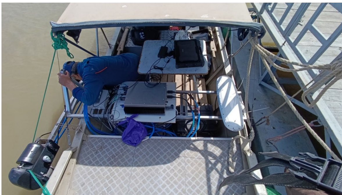
Figure 3. The Geoswath 4r mounted on a small survey boat
