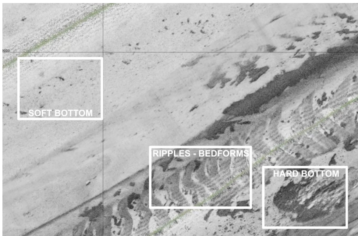
Figure 2. Sidescan image generated by interpreting the backscatter data collected by the GeoSwath 4R sonar.
